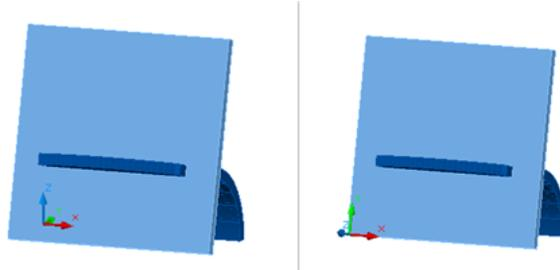
The left image shows the user coordinate system not aligned to the face plate of the 3D object and the right image shows the user coordinate system aligned to the face plate of the 3D object.
