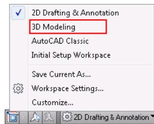
The 3D Modeling workspace is displayed. The Workspaces icon in the status bar indicates that you are now in the 3D Modeling workspace. In this workspace, you can access the various commands and tools needed for creating 3D drawings.
